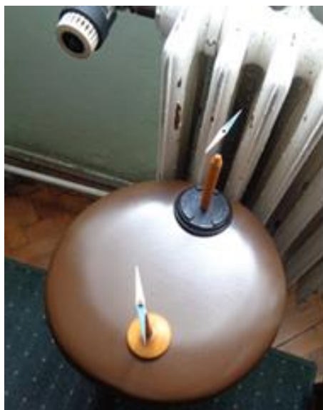
Fig. 2: The deviation of the compass indicates magnetisation of the cast iron radiator.
