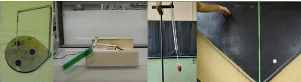
Fig. 1: Simple chaotic tools (from left to right): magnetic pendulum, driven pendulum, elastic pendulum, and ball bouncing on double slope used in the introductory, experimental part of the teaching module (photos taken by the author).
